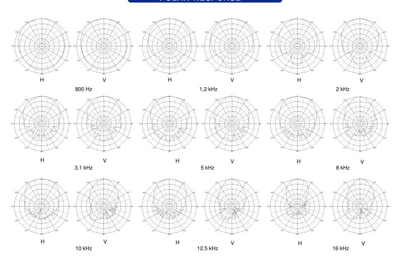
\*Horizontal beamwidth is represented by the heavy line. Vertical beamwidth is represented by the discontinuous line.
