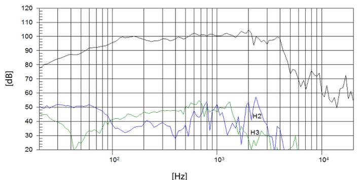
Note: On axis frequency response measured with loudspeaker standing on infinite baffle in anechoic chamber, 1W @ 1m
