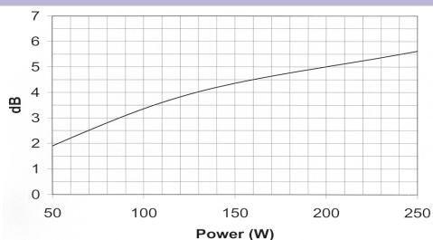
Note: These losses are calculated from a five minutes AES power test applying band limited pink noise (120-3500 Hz). The loudspeaker is free-air standing.
