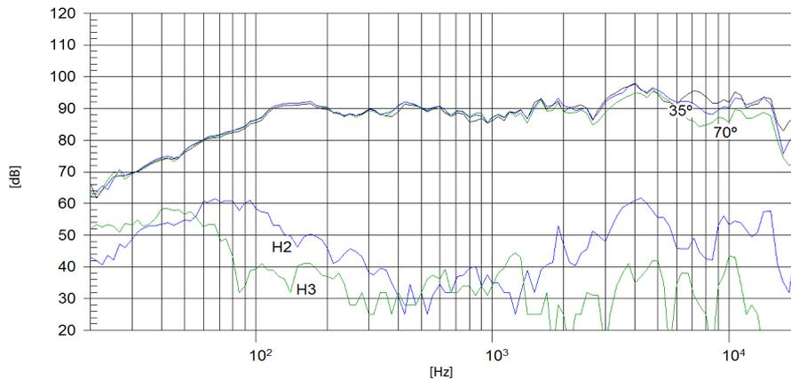
Note: Filtered frequency response measured with loudspeaker standing on infinite baffle in anechoic chamber, 1W @ 1m with FD-2CX/Fe
