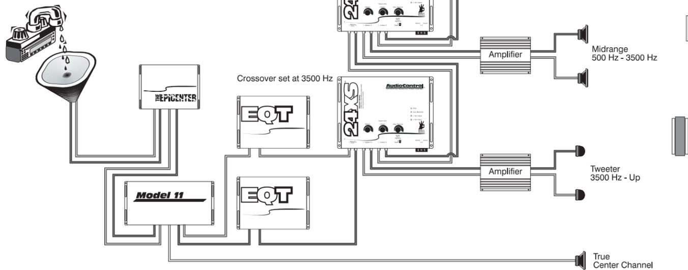
The Speaker Wave Alignment Technology (SWAT) in your 24XS shifts the output of the crossover slightly so you can move the dead zones in the sound pattern away from the listener's ears. This tilting will always go towards the output that you have selected with the internal switches on the 24XS. See the next section on adjusting the Speaker Wave Alignment control for more information.
